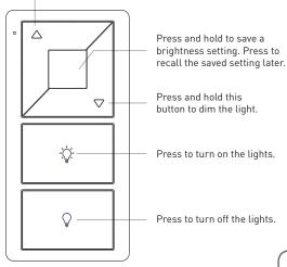
SlimDim Wireless Dimmers are a revolution in lighting control. Using long range RF technology, these dimmers avoid the need for connecting directly to a power supply, cutting down on cost and installation time. SlimDims are simple and quick to install.
